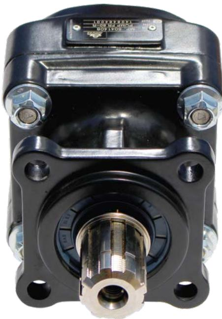
This hydraulic pump is a bent axis type pump with fixed displacement, developed under the design of spherical head pistons. This gives to the pump a very high performance and high pressure ratings on a long life span unit with European standard assemblies. Therefore, this pump can be mounted directly in most of PTO's in the world.
