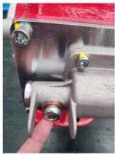
Remove the plug from the indicator switch port of the pneumatic shifter housing.
