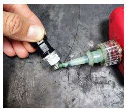
Apply a few drops of Loctite 270 to the new indicator switch thread.
