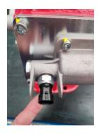
5. Fit the copper washer into the switch and tight it (30Nm / 22Lb.ft) to the cover.
