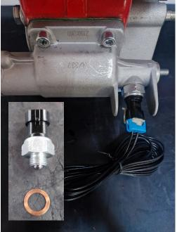
4. Fit the copper washer into the switch, tight the new indicator switch (30Nm / 22Lb.ft) and plug the wire.
