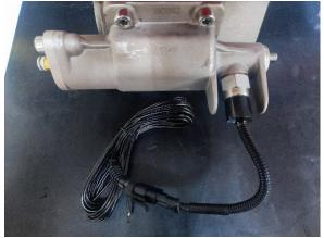
1. Unplug the wire and remove the indicator connector from the pneumatic shifter housing.
