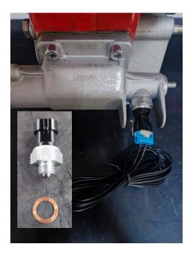
4. Fit the copper washer into the switch, tight the new indicator switch (30Nm / 22Lb.ft) and plug the wire.
