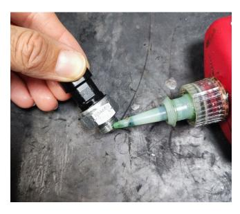
Apply a few drops of Loctite 270 to the new indicator switch thread.
